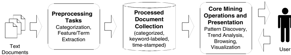
Figure I.4. High-level text mining functional architecture.
